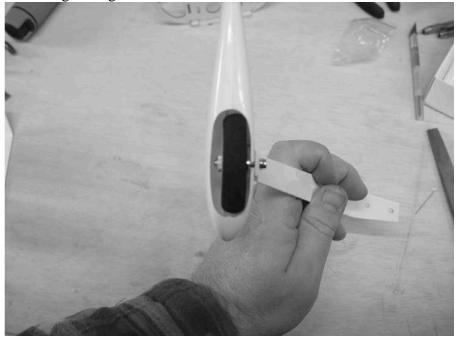
7. Insert the gear legs through the slots and retain with the (4) 3mm bolts and washers. Make sure to put a drop of blue Loctite on the bolt threads. The gear legs should sweep toward the rear of the plane.
