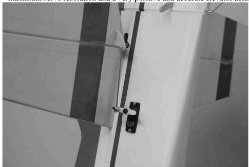
19. Use a #11 blade to remove the covering from the rudder control horn slot near the bottom of the rudder. Locate the composite control horn for the rudder. Scuff the control horn to remove the glossy finish and glue into place in the slot in the rudder. Assemble the pushrod
