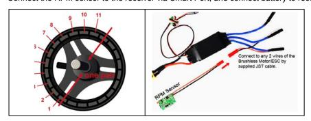
3. Long pressing the Key until the RED LED Soiled ON to enter Pole Pairs setting mode. Set the number on the RPM sensor by push the key repeatedly until you've got the correct number (The Digital number is Binary value, see below chart for details).
