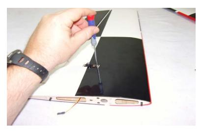
7. Locate the 2 threaded pushrods that are the same size and 4 micro ball links along with 4 2mm screws, nuts and washers. Thread the ball links onto each end of the pushrods and secure to the servo arm and control horn with the 2 mm hardware as shown in the picture. Use the longest arm provided with your servo.
