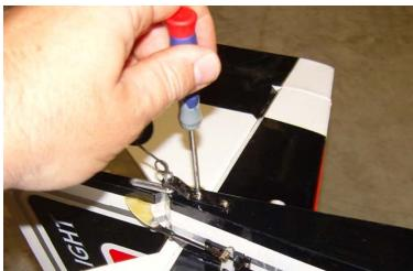
16. Secure the tiller using the provided screw, but do not over tighten as the tiller should be able to move on the screw as the rudder is deflected.
