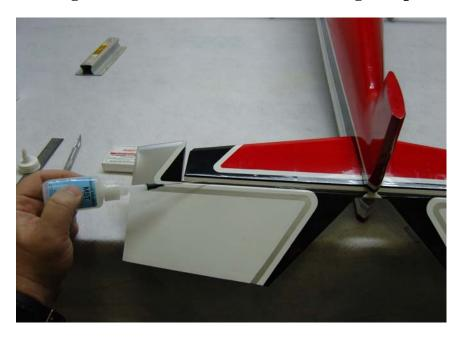
13. Remove the covering over the slot in the lower right side of the rudder where the rudder control horn will be installed. Scuff the portion of the control horn that will glue into the surface and secure the rudder control horn with medium CA.
