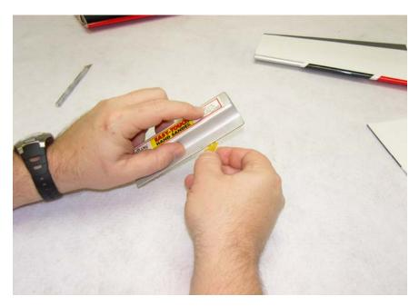
3. Use a glue tip on your bottle of medium CA and apply glue to the slot as well as to both sides of the control horn. Insert the control horn into the slot and make sure it seats properly against the surface of the aileron.
