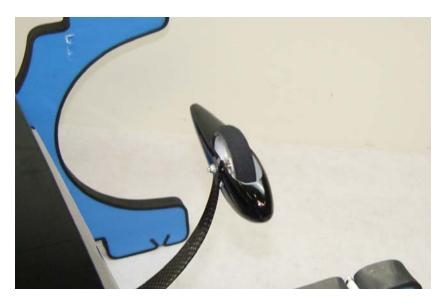
10. Locate the horizontal stabilizer/elevator assembly and slide the elevator off of the hinges. Insert the stabilizer into its slot and the carbon fiber wing tube into the fiberglass sleeve. Use a ruler to insure that the stabilizer is centered in its slot and compare the stabilizer to the wing tube to make sure it is properly aligned. Sand or shim the slot if necessary to ensure proper alignment. Secure the stabilizer with CA.
