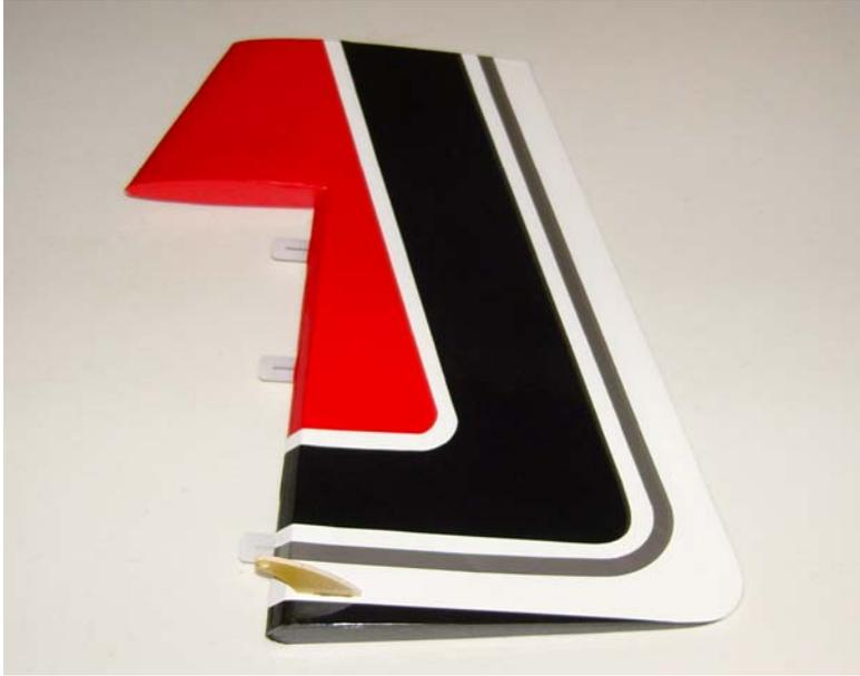
**19. Using the same process as with the ailerons and elevator, slide the rudder onto the hinges and secure to the vertical stabilizer with thin CA.**
