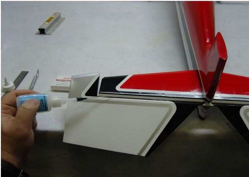
**18. Remove the covering over the slot in the lower left side of the rudder where the rudder control horn will be installed. Scuff the portion of the control horn that will glue into the surface and secure the rudder control horn with medium CA.**
