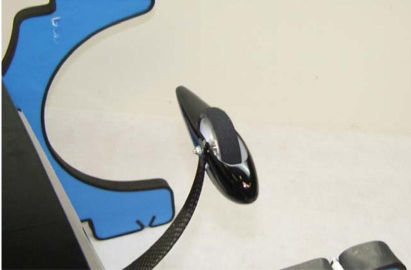
**15. Locate the horizontal stabilizer/elevator assembly and slide the elevator off of the hinges. Insert the stabilizer into its slot and the carbon fiber wing tube into the fiberglass sleeve. Use a ruler to insure that the stabilizer is centered in its slot and compare the stabilizer to the wing tube to make sure it is properly aligned. Sand or shim the slot if necessary. Secure the stabilizer with CA.**
