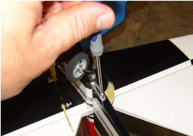
**22. Place the tailwheel wire in the proper position, aligned with the rudder and lock into place with the 2 set screws.**
