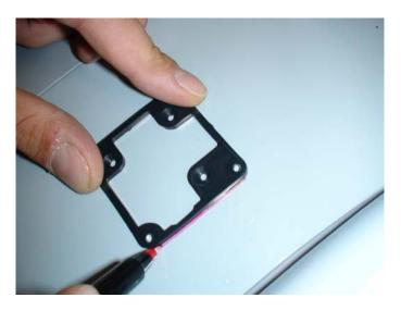
5. Using a scalpol, carefully cut, following the inside of the line. If you are cutting in to a solid material then only cut to the depth required to fit the frame flush with the surface of the aircraft.
