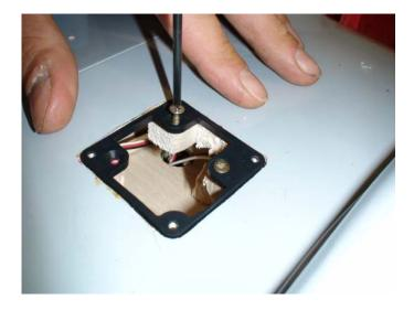
14. Pass the servo leadthrough the hole and connectit to your receiver orsequencer.Then using the countersunkscrews provided, fix the frontplate to the frame.
