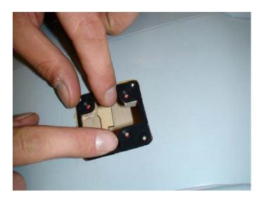
13. Using small countersunkscrews or cuntersunk bolts,secure the frame in position.Take care to ensure that theheads of your screws to not sitabove the surface of the frame.
