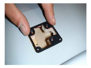
11. Using a 3mm drill bit, make holes through the wood at each corner where you have made marks. These will allow the front plate countersunk screws to pass through when tightened.
