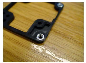
3. Place the frame on the surface on which you would like to locate your **BOMBS AWAY** Take care to ensure that the nuts are facing away from you and the two offset countersunk holes are towards to front of the aircraft.
